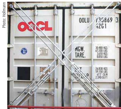
PROTECTION. On the bottom tiers, containers are reinforced by bolted-on cross braces made of high-strength steel.
