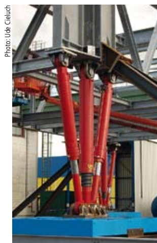
TECHNIQUE. The hydraulically-operated posts.
