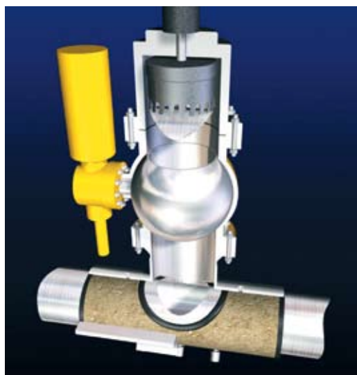
COVER INSTEAD OF WELDING: The "Grouted Tee" is an example of the creativity of Advantica's engineers.
