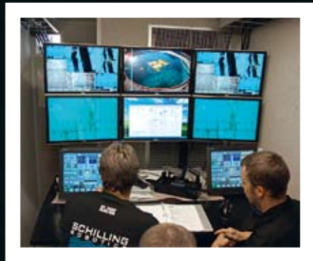
CONTROL CENTRE. From the parent ship all ROV functions can be steered.
