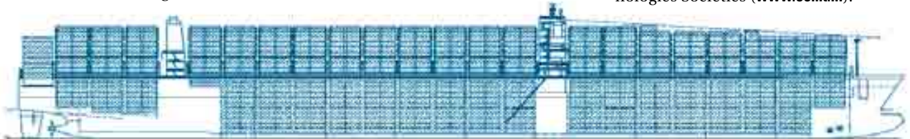
STUDY. 366 metres in length, 48.2 metres in breadth: the designed 13100-TEU giants designed from Hyundai Heavy Industries.
