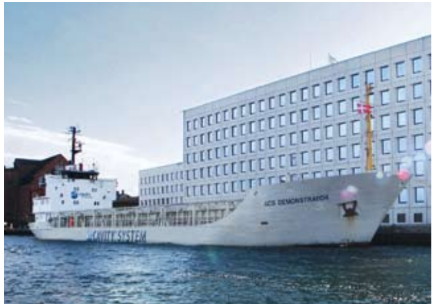
ACS DEMONSTRATOR: A coaster built in 1980 is being retrofitted with the Air Cavity System by the Dutch DK Group ( www.dkgroup.eu ).
