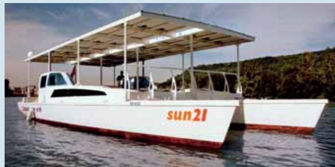
SOLAR DECK. The solar catamaran is powered exclusively by solar energy.
