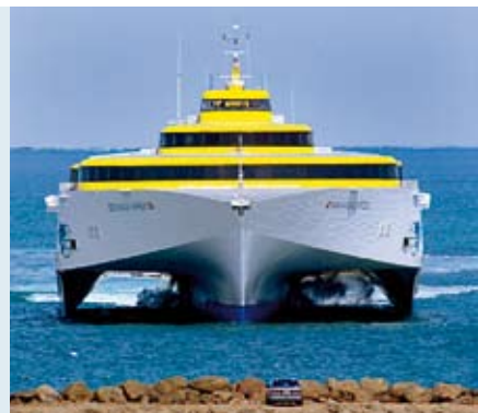
LIGHTWEIGHT CONSTRUCTION. The fast trimaran "Benchijigua express" consists entirely of aluminium.
