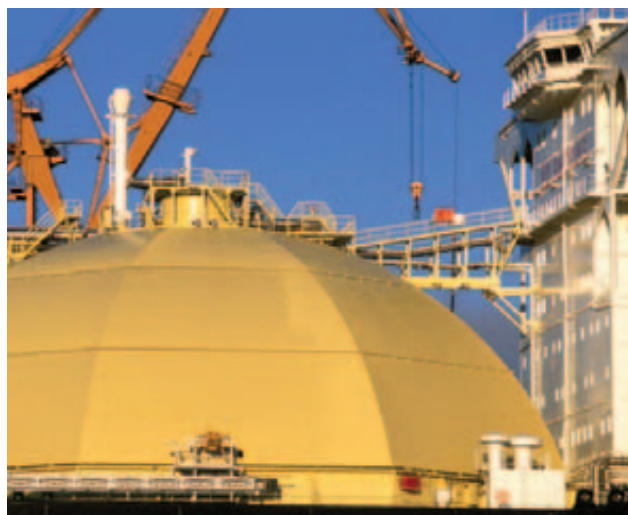
With the Moss tankers, the aluminium containers only need a wall thickness of 4 cm, thanks to their spherical shape
