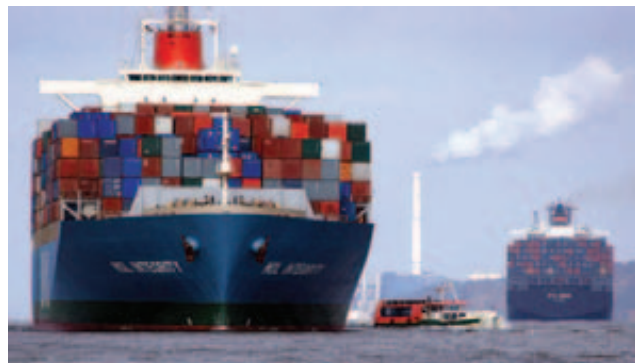
Containers are stacked up to eight tiers high on deck
