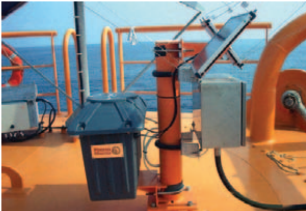
Datalogger and power supply to record the load data
