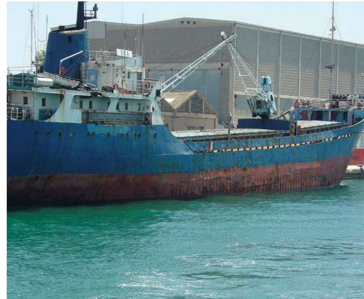
Rust bucket in the port of Barcelona: ecological anti-corrosion coatings are to be used increasingly in future
