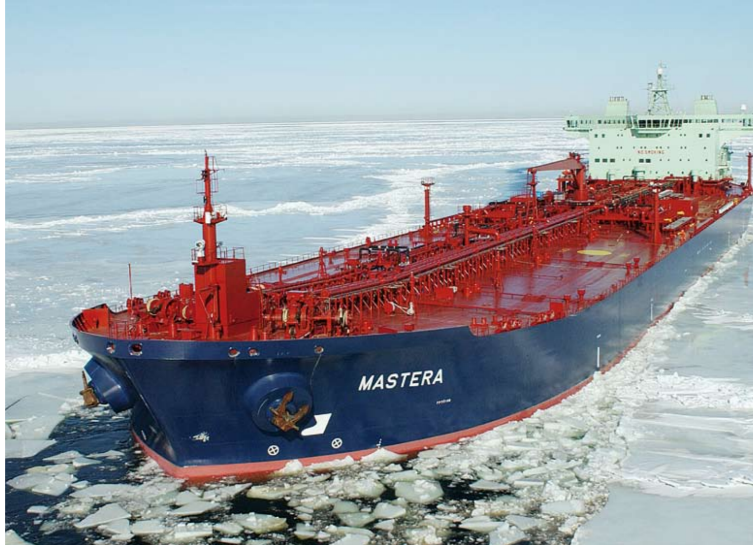
The crude oil tanker "Mastera" needs no icebreaker because it has a high ice class
