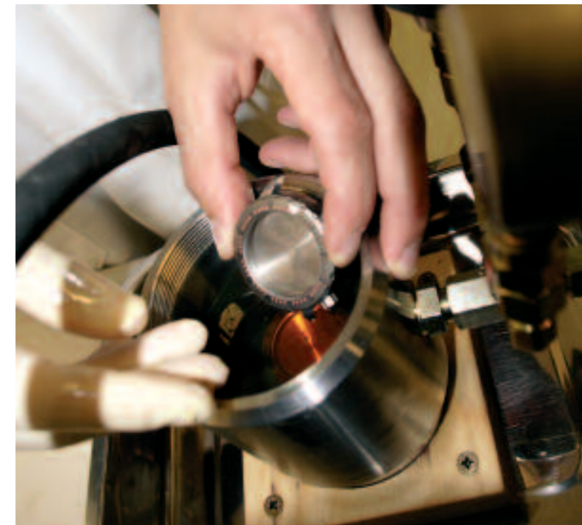
Certified by Germanischer Lloyd: the U2 (top), made of submarine steel, is available now. Below: Part 1 of the test, in which the watches are lowered into the special pressure-testing chamber
