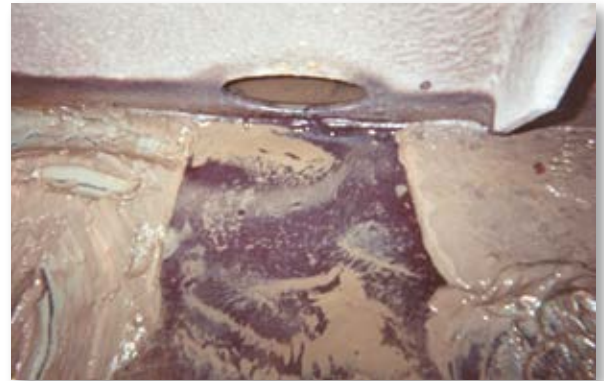
FIGURE 2. Sediments accumulate in ballast water tanks in areas with flow stagnation.
