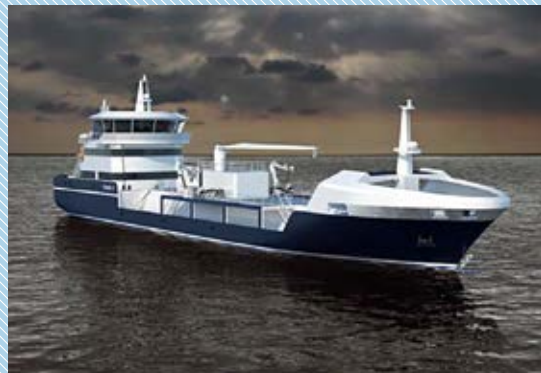
FKAB. This vessel will be equipped with two engines capable of burning either LNG or biogas.
