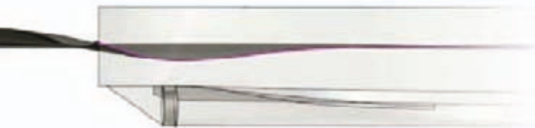
AFTERBODY. Wave pattern – Postmodel02.3
