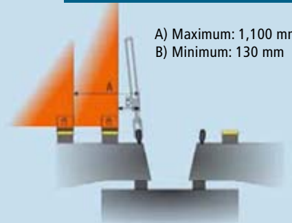
FIG. 1. Distance lashing eye – container on deck/hatch cover
