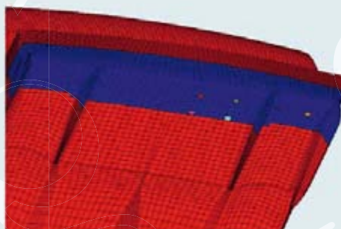
STERN OF A MEGAYACHT. Original design (left) and modified design for reduced slamming impact (right); slamming pressures were reduced by almost 30 per cent.
