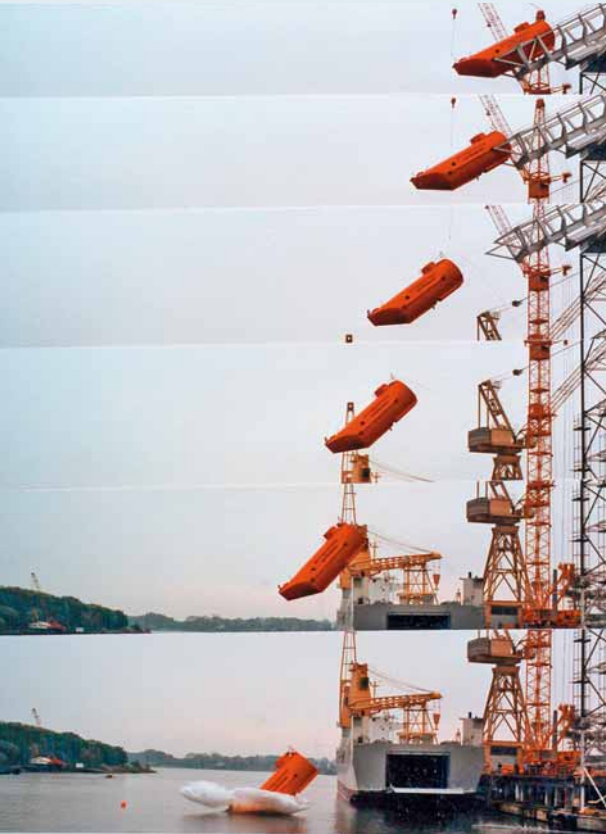
EFFORT. Test of a lifeboat at a free fall from a very high ramp.
