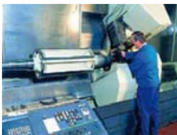
TECHNOLOGY. Machining a shaft from all sides in one step.
