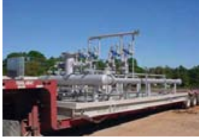
TRANSPORT BY LAND. Large assemblies are carried on special low-platform trailers.
