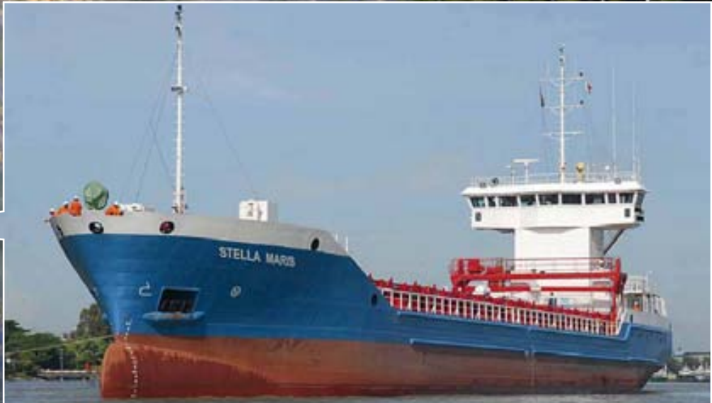
PIONEER. "Stella Maris" by ASSL. The data: length over all 81.35 metres, breadth moulded 13.15 metres, depth moulded 6.20 metres. MAN B&W 8L21/31 engine (output 1,720 kW), CPP. The assigned class notation for the vessel is as follows: hull: + 100 A 5 E with freeboard 1.560 metres; SOLAS II-2 Reg 19 DBC; multi-purpose-dry cargo ship; equipped for carriage of containers; strengthened for heavy cargo. Machinery: + MC E AUT-16h.
