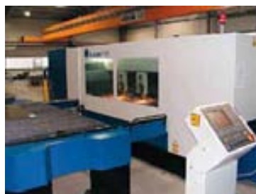
PRODUCTION. Ultramodern dual-head laser cutter for electrical sheets.
