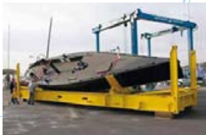
PRECISION WORK. The open 40-foot box was designed and built for the transport of the one-design class RC 44.
