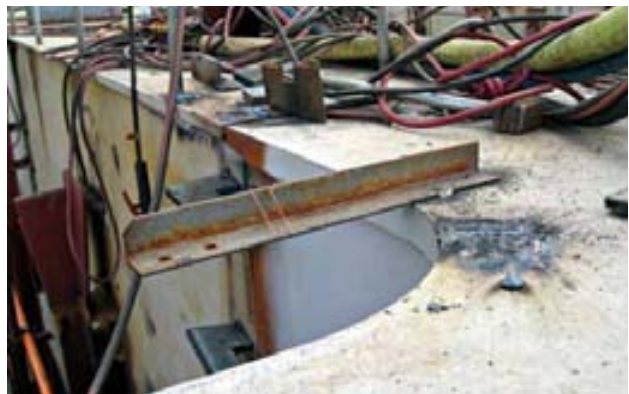
HATCH CORNER. This is an area subject to high stress. Welding should be avoided if possible.
