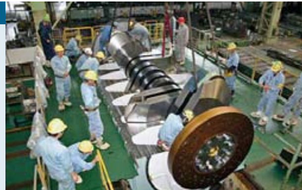
PRODUCTION. Crankshaft of a two-stroke engine fitted with a Geislinger vibration damper.
