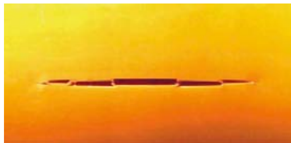
Figure 4. Brittle failure of PE pipe – slit type fractures.
