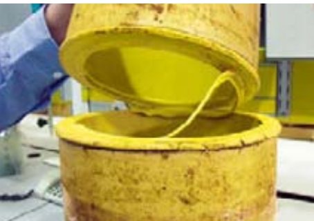
Figure 6. Catastrophic failure of a butt fusion joint.
