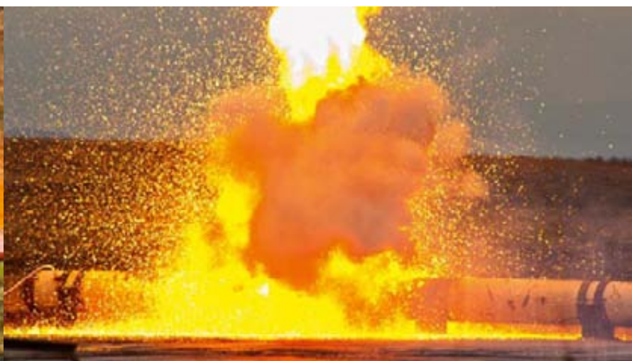
Demo. An attack on a steel pipeline conveying propane at two bar.
