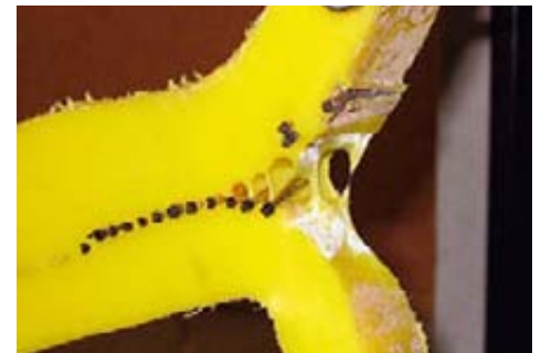
Figure 8. Tensile testing of an electrofusion weld specimen.
