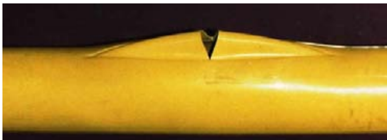
Figure 3. Ductile failure of PE pipe under internal hydrostatic pressure.
