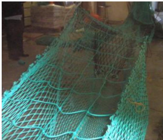
Boxed extension section showing large square mesh in the top and smaller diamond mesh in the sides and bottom panel
