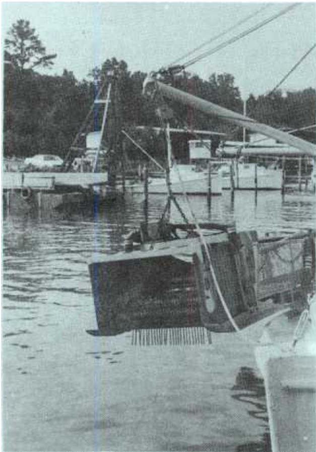
The harvester head consists of a steel box with rows of flexible steel tines affixed to two cylinders.
