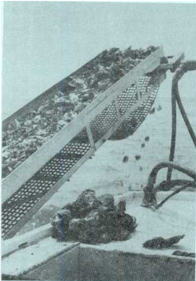
Unwanted shell moves along the escalator and falls back to the bottom.
