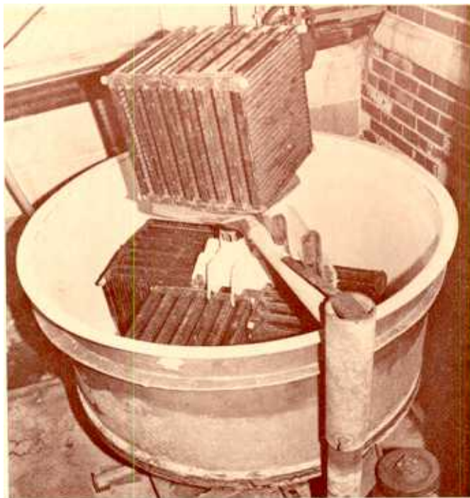
Invented by Dupuy to complement the French grid collector package for hatchery use, this rotating tank for setting larvae precludes the setting of spat on the tank surface.
