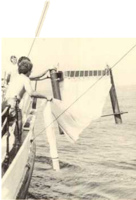
The "Neuston Sampler," designed by the ODU blue crab research team specifically for sampling the ocean's neuston layer, is brought aboard by ODU graduate students operating the device in Chesapeake Bay waters.
