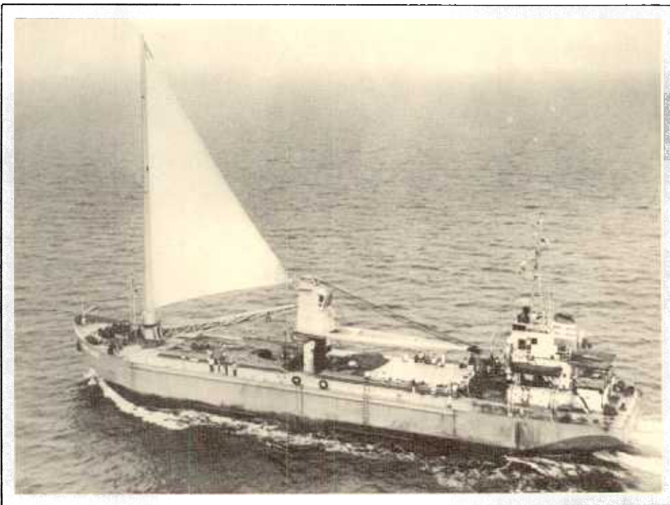
The Greek cargo ship MINI LACE is working out of New Orleans in the Caribbean tramping trade. Her 214' length is helped along by a fully automated sail, providing fuel savings.
