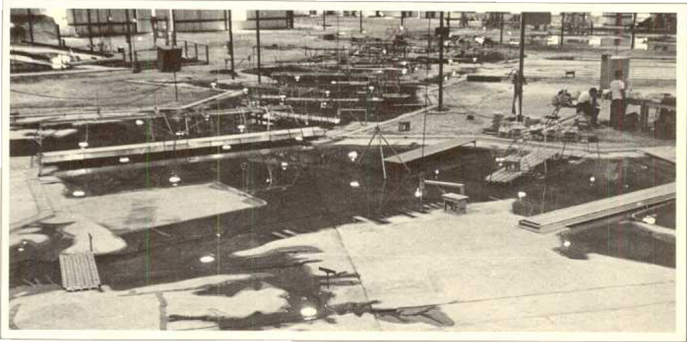
This is only a part of the U.S. Army Corps of Engineers Chesapeake Bay hydraulic model, housed under one 14-acre roof at Stevensville, Maryland. Drs Blair and Hecker hope it can aid efforts to update marina buffer zones in Virginia.
