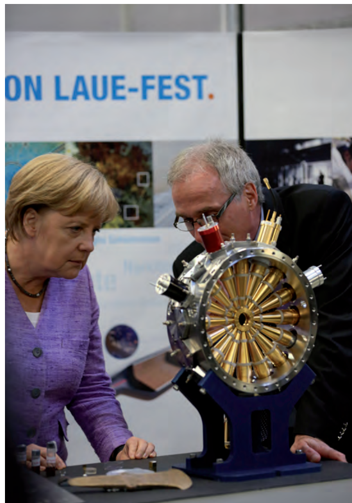
Figure 2 View inside the diagnostic unit. German Chancellor Angela Merkel and DESY Director Helmut Dosch are inspecting the 16 independent drift tubes of the electron time-of-flight spectrometers.
