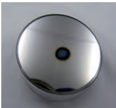
Figure 3 Carbon contaminated off-axis parabola.
