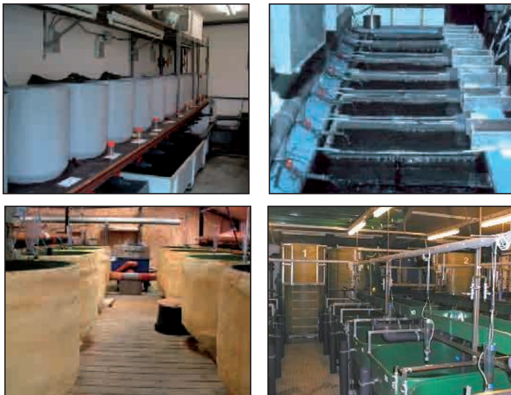
Plate 5.5: Clockwise from top: cylindro-conical tanks and tank-based cages used for the experimental culture of perch larvae in recirculation aquaculture system (CEFRA, University of Liège, Belgium). squared tanks for production of weaned juveniles used at Bornholms Hatchery (Denmark). cylindro-conical tanks for incubation and early rearing of perch.
