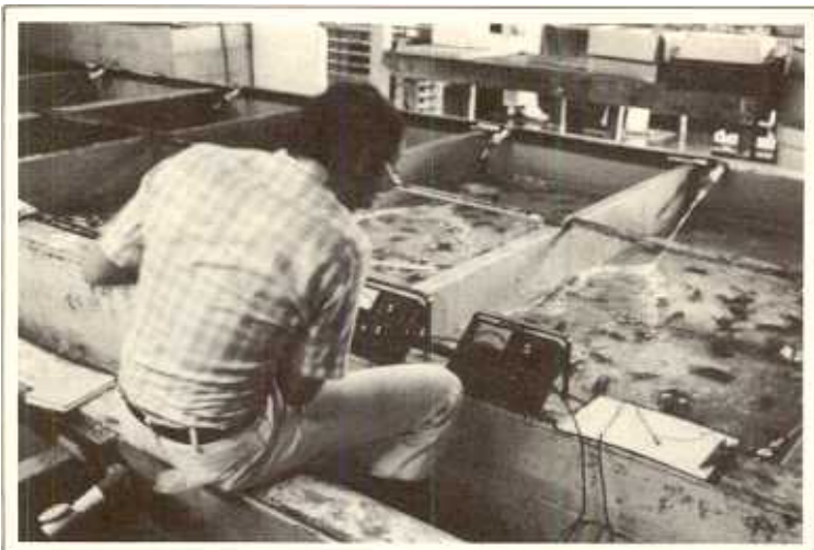
VIMS commercial fisheries specialist Mike Oesterling monitors oxygen and pH of the water in Lewis Whittaker's closed design crab shedding operation.
