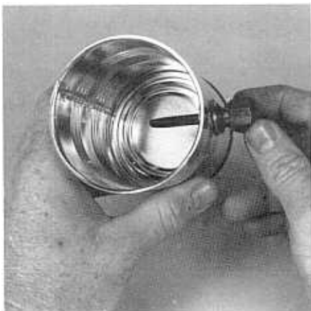
Installation of a thermocouple in a metal can to enable plant managers to verify internal temperature of pasteurized crab meat.
