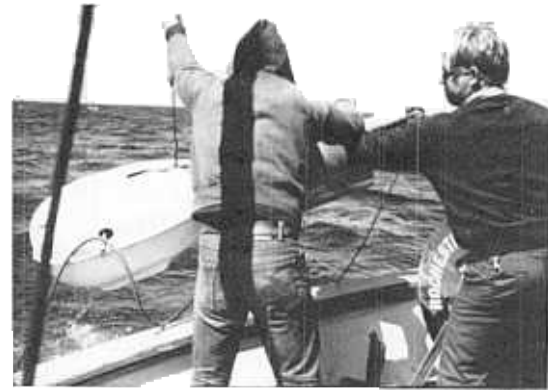
Dr. C. R. Berquist (r) and assistant drop the seismic "fish" over the side of the research vessel. Berquist will examine the resulting readings for indications of likely mineral deposit sites.
