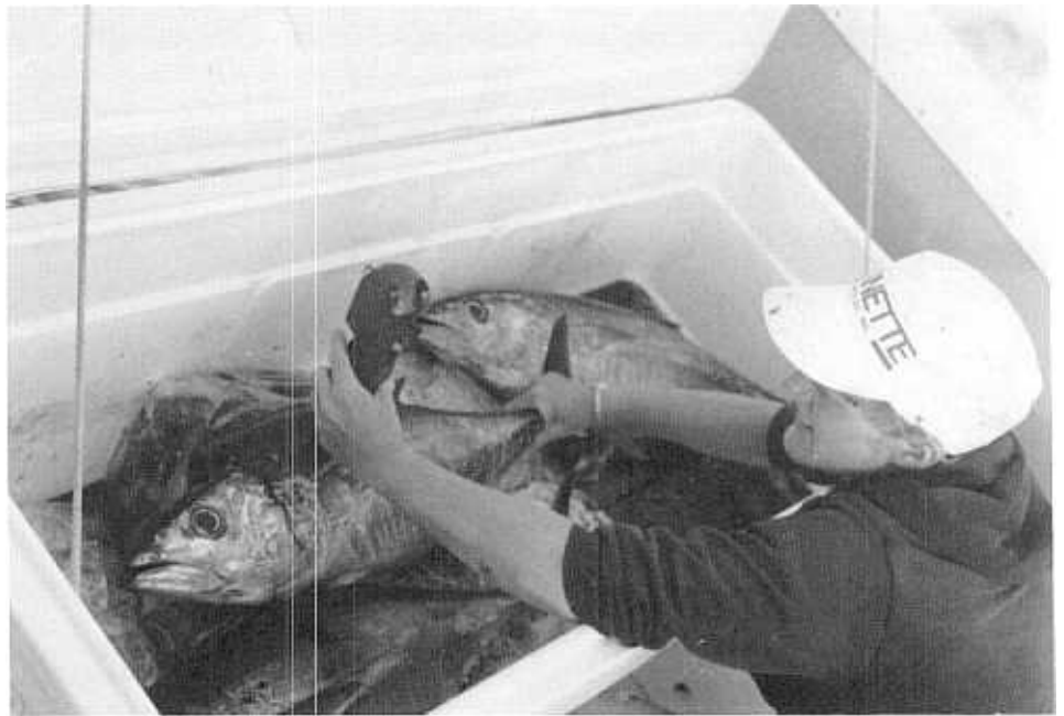
Nancy Chartier, VIMS' graduate student is using a Torrymeter which measures characteristics of the tuna skin and muscle tissue as an indication of freshness.
