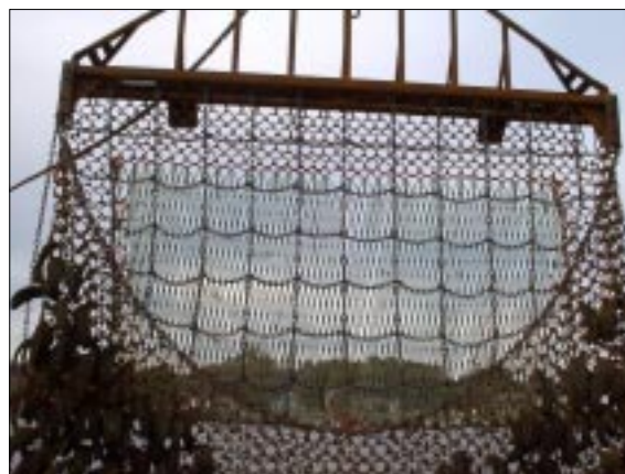
The modified dredge shown above is designed to keep sea turtles out.
