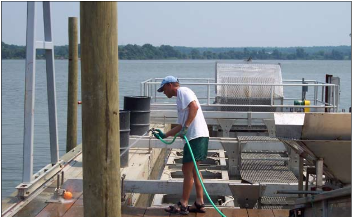
Aquaculture has increased about 10-fold since industry trials with non-natives began. Some growers have scaled up in anticipation of triploid aquaculture by investing in infrastructure like the floating upweller system shown above. Here, A.J. Erskine (former project manager for the VSC trials), cleans upwellers for the joint-venture operation located in the Coan River.
