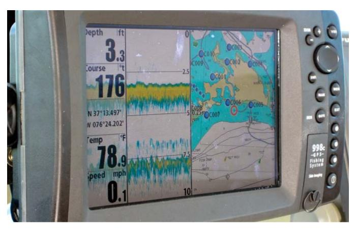
The screen on Zimmerman's sonar and GPS chartplotter displays the vessel's GPS location and the depth of the water. This bathymetry data will be used in generating a model of potential seagrass distribution.
