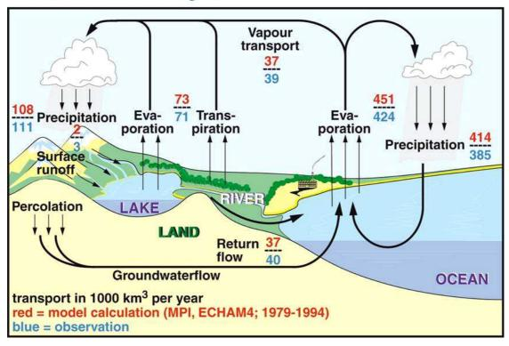
**Figure 1** Global water cycle with flux estimates based on the GCM ECHAM4 (*Roeckner et al.* 1996) for the period 1979-1994 and climatological estimates of *Baumgartner and Reichel* (1975). Unit: 1000 km<sup>3</sup>/a.
