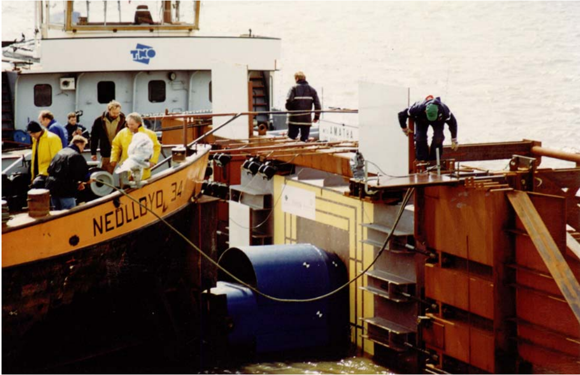
Figure 1 Ship to Ship Collision Test
