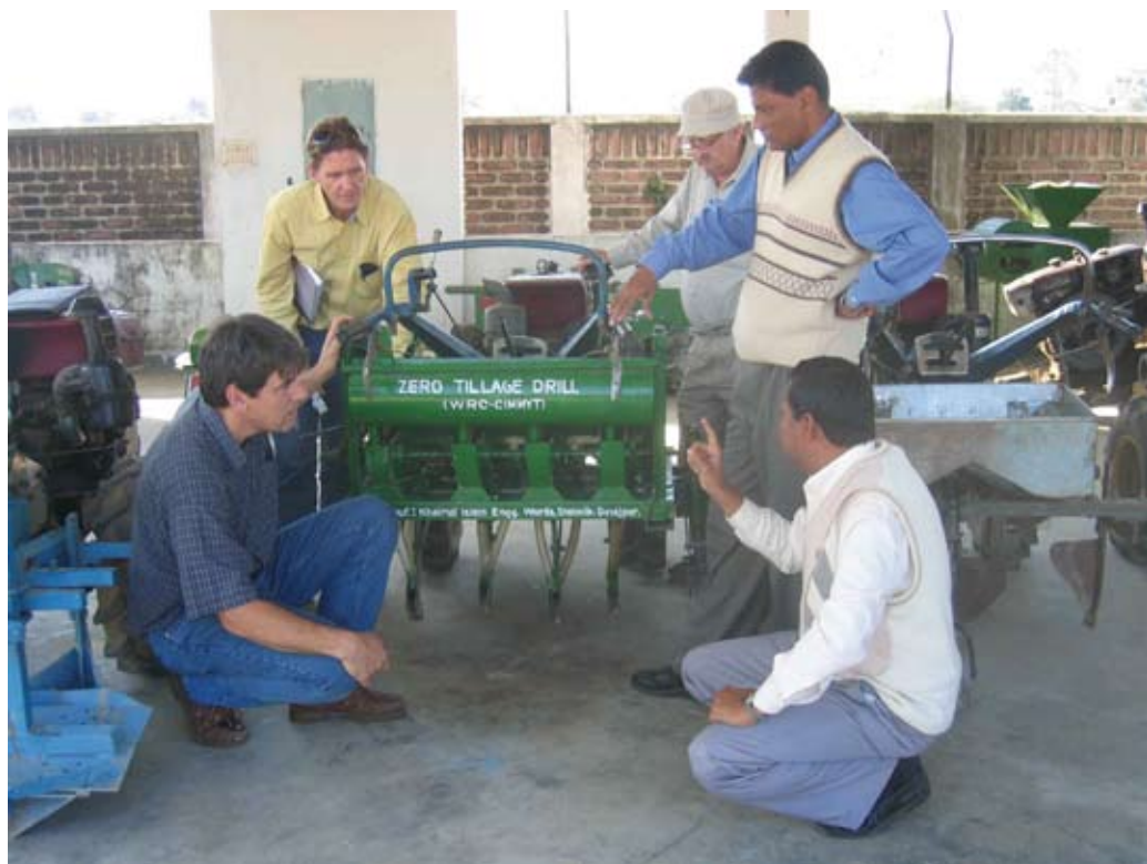
A locally manufactured power-tiller, zero-till drill
