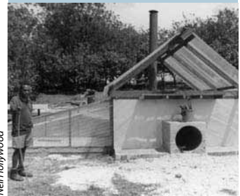
A combination solar kiln dryer developed for cocoa in PNG
