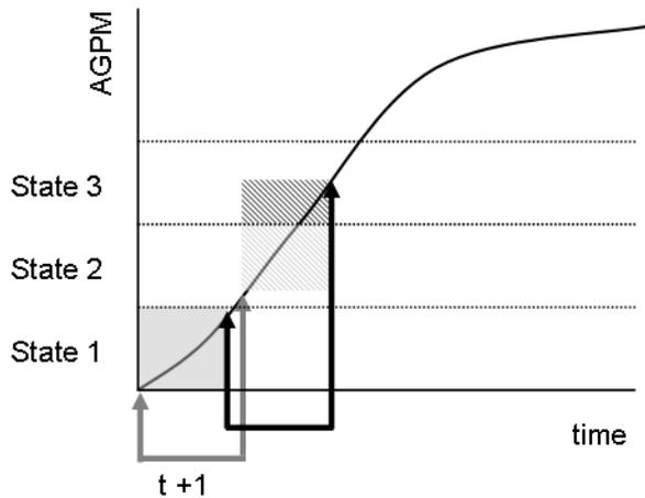
**Fig 4** Determination of transition probabilities between states of AGPM for a given HRU, management and climate regime. AGPM is displayed against time. Grey arrowed lines measure one time step starting from the lower boundary of vegetation state 1, and black arrowed lines measure one time step starting from the upper boundary of vegetation state 1. Heights of the shaded squares indicate the range of possible vegetation states after one time step.
