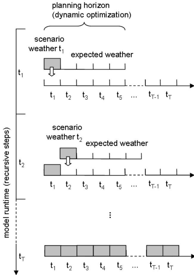
**Fig 2** Mixed recursive-dynamic LDM with a planning horizon of five years. The indices  $t_1$  to  $t_T$  represent individual years of the entire model runtime. Grey boxes represent the results of the first years of dynamic optimization, which are used as initial conditions for the next time step and results of the recursive model.
