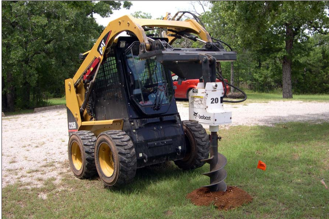
Figure 11. Caterpillar Bobcat 226B with front-mounted auger drilling a test at Guy Sandy Campground West.
