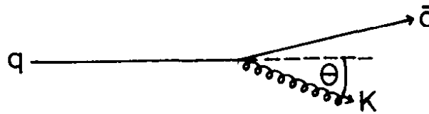
Fig. 41 Illustration of the process e^+e^- \rightarrow q\bar{q}g
