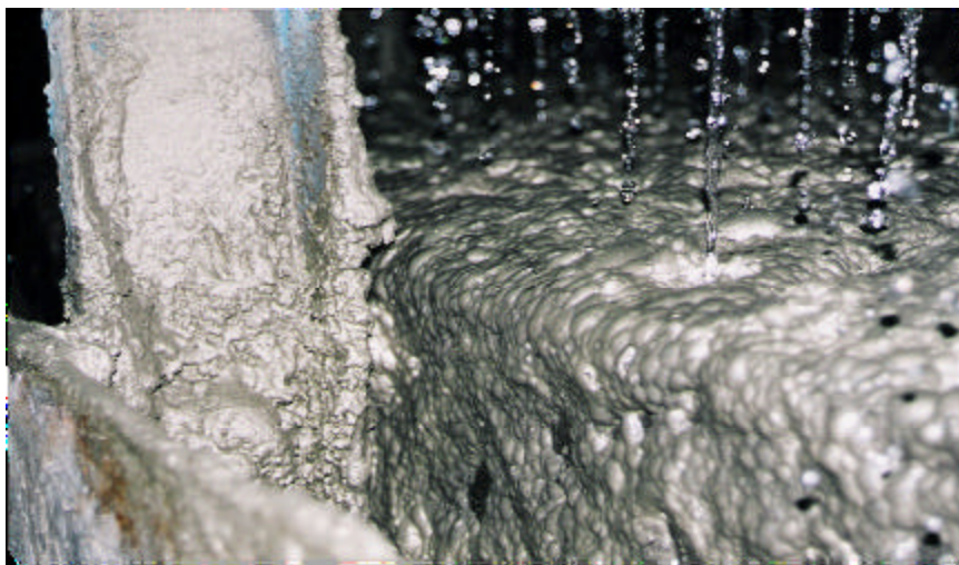
After the ore is ground into a fine powder, the floatation process brings the target minerals, such as copper, to the surface of the fluid in the form of bubbles. This separates the target mineral from the unvaluable materials, the tailings. The bubbles are skimmed off and dewatered to create the concentrate that will be transported from the mine site. The tailings are piped to the tailings impoundment area for permanent storage. (Photo: Huckleberry Mine, BC. C. Slanina, 2005)
