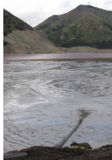
Tailings pumped into tailings impoundment area at Kemsess South Mine. (Photo: C. Slanina, 2007)
