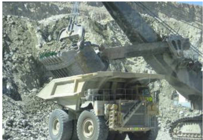
In an open pit mine, this electric shovel puts ore into a haul truck. (Photo: Sierrita Mine, AZ. C. Slanina, 2007)
