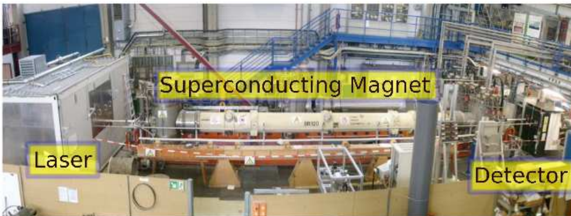
Figure 6. The ALPS experiment at DESY [61,62]. The primary laser system is kept in a light tight hut in the left hand side. From it, laser light is injected in the bore of a HERA superconducting dipole magnet. A blocking wall is placed in the center of the magnet's inner bore. Light eventually regenerated behind the wall would continue its trip through the magnet to end up in a black cabinet enclosing the photon detector.
