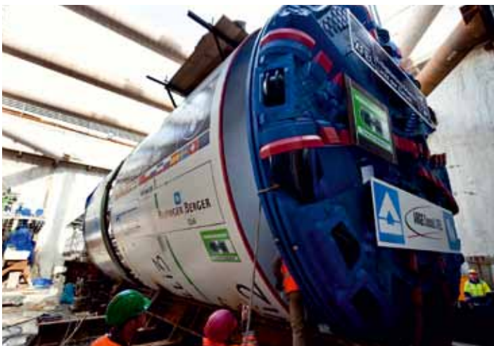
Assembly of the first European XFEL tunnel boring machine. (Photo: European XFEL)
