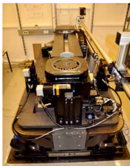
Figure 3 Microtomography set-up installed at the Imaging Beamline IBL (P05 at PETRA III). An almost identical set-up has already been installed at HEMS (P07) as well.
