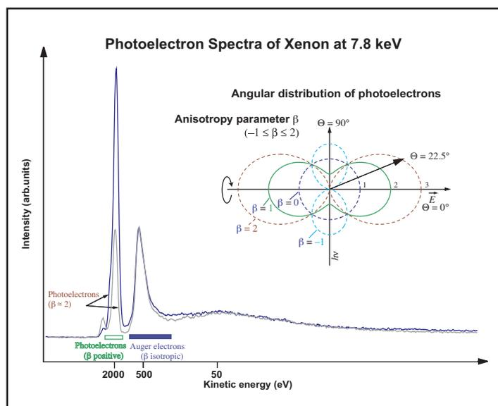
**Figure 3** Photoelectron spectra of Xenon at a photon energy of 7.8 keV. The dark blue curve and the light grey curve show the 22.5° and 90° time-of-flight detector signals, respectively. Angles are measured relative to the horizontal direction. The ratio between the photoelectron peaks of both detectors points to a positive  $\beta$  of about 1. The outer areas of the photoelectron peak (accented) show a  $\beta$  of almost 2.
