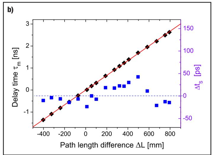
b) Left axis: Measured delay time vs. path length difference  $\Delta L$ . The red solid line denotes a linear fit to the data. Right axis: The difference between expected and measured delay time is quantified by the blue squares.
