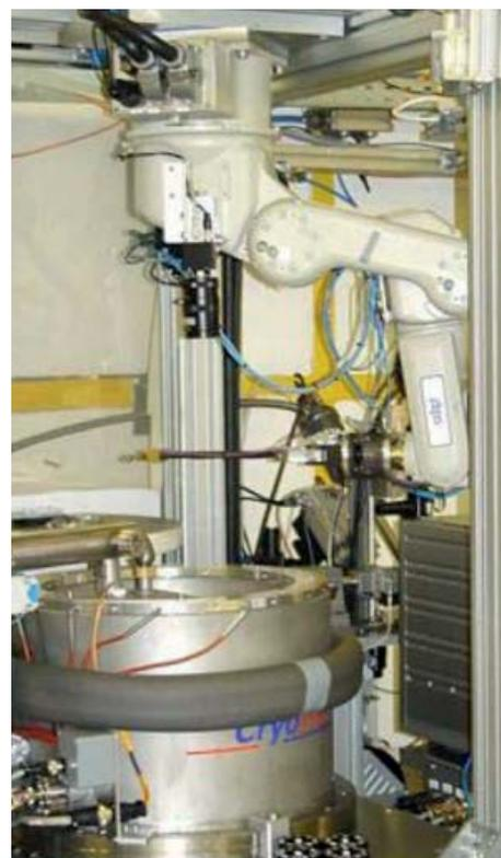
crystallography beamlines - have arrived. They have been initially installed on the DORIS wiggler-beamline BW7A for testing. In preparation for the future facilities at PETRA III, this beamline is now fully controlled by the TINE control system with an mxCube (ESRF) based graphical user interface. Many test data sets have been successfully collected using this prototype setup. An in-house development for a new sample changer
