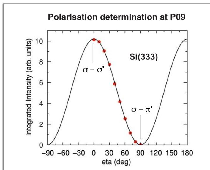
**Figure 4** Polarisation dependence measured at 7.83 keV at the P09 beamline on the Si(333) reflection using a pyrolytic graphite crystal as polarisation analyser.
