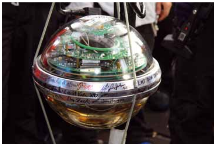
The last digital optical module (DOM) is being deployed in the IceCube detector.
