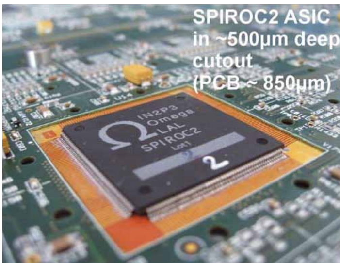
Figure 2 Calorimeter readout ASIC for 36 silicon photomultiplier channels, embedded in a printed circuit board optimized for compactness
