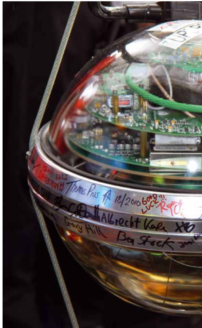
The last digital optical module (DOM) is being deployed in the IceCube detector.
