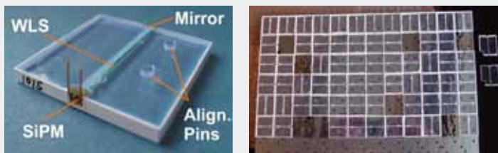
Figure 1 A scintillating tile with SiPM (left) and assembled tiles on a calorimeter readout layer (right)
