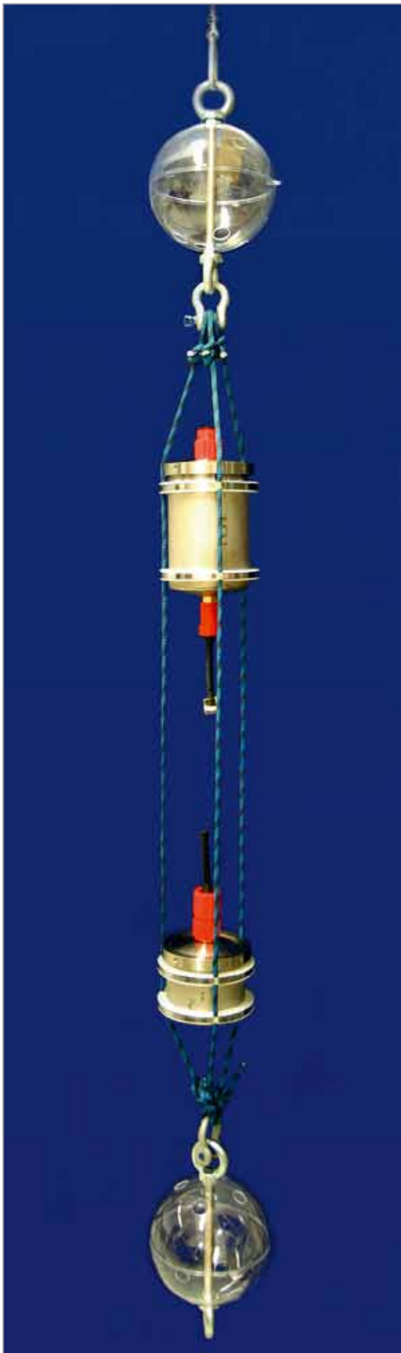
Figure 2 SPATS acoustic station
