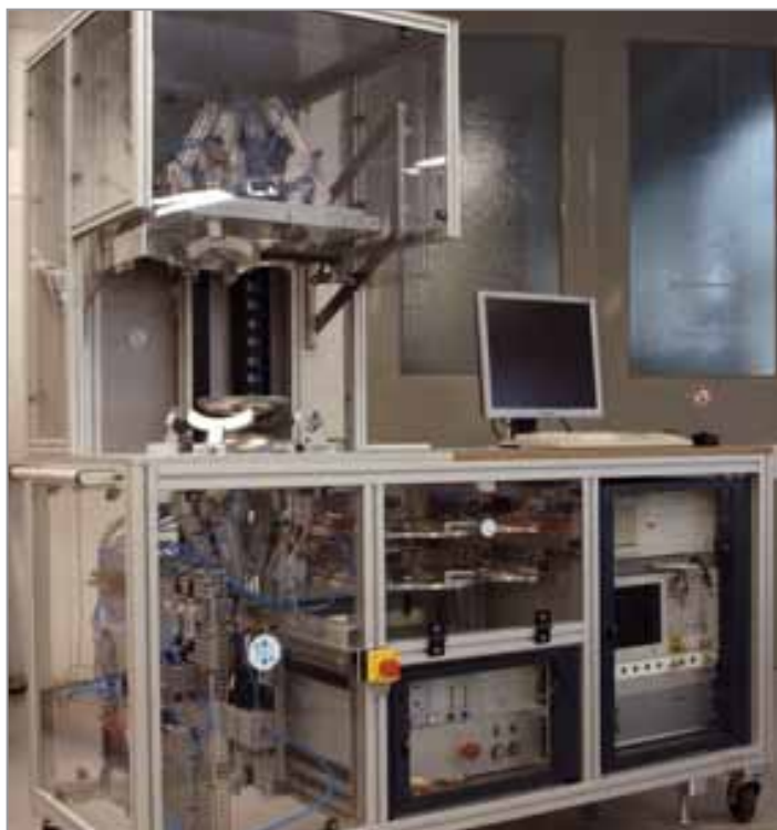
Figure 2 The machine and controls for measuring the RF performance of cavity half-cells (HAZEMEMA) [1]. The protocols are automatically registered and recorded.
