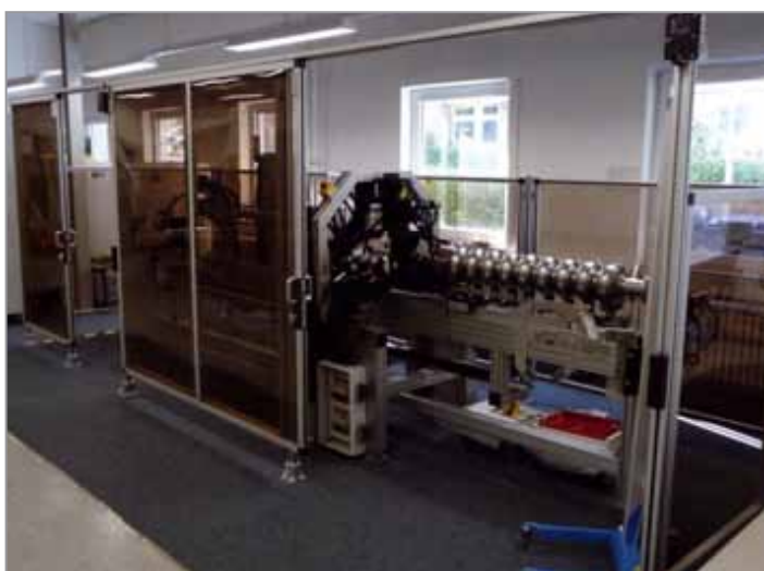
Figure 3 The tuning machine [2] that mechanically adjusts the size of individual cells to meet the stringent resonance requirements of the accelerator. The adjustment is done fully automatically, thus increasing reproducibility and reducing cost.
