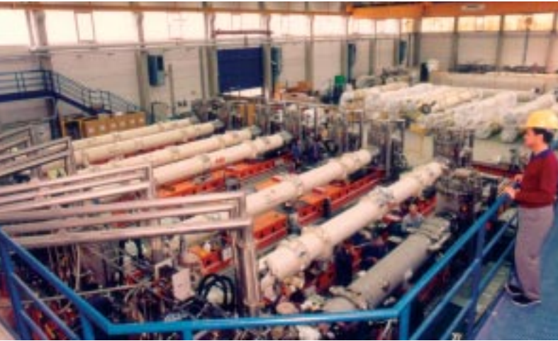
Test of the superconducting proton magnets for HERA.
