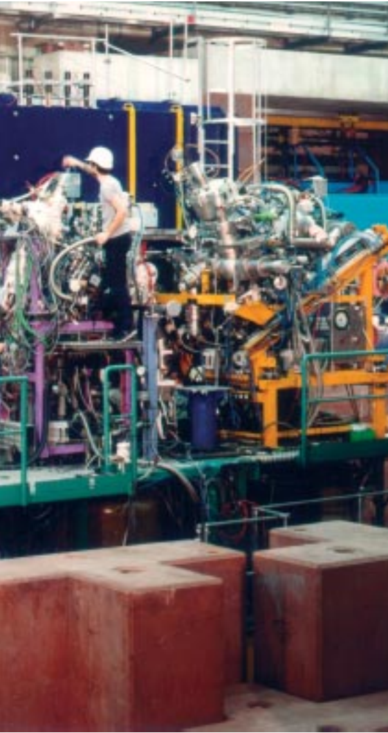
The HERMES detector in HERA's East Hall: In the foreground is the gas target area, behind it the large spectrometer magnet (blue).
