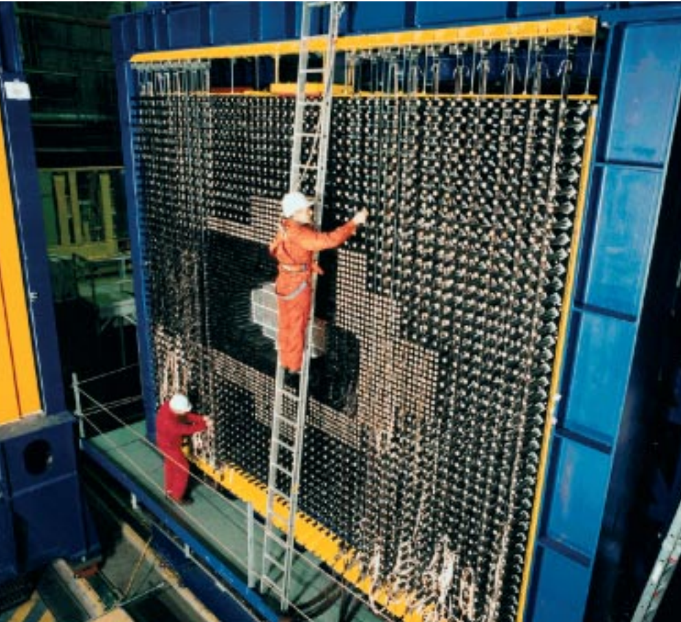
Particles are captured and identified in HERA-B's electromagnetic calorimeter, which is five meters high and six meters wide.
