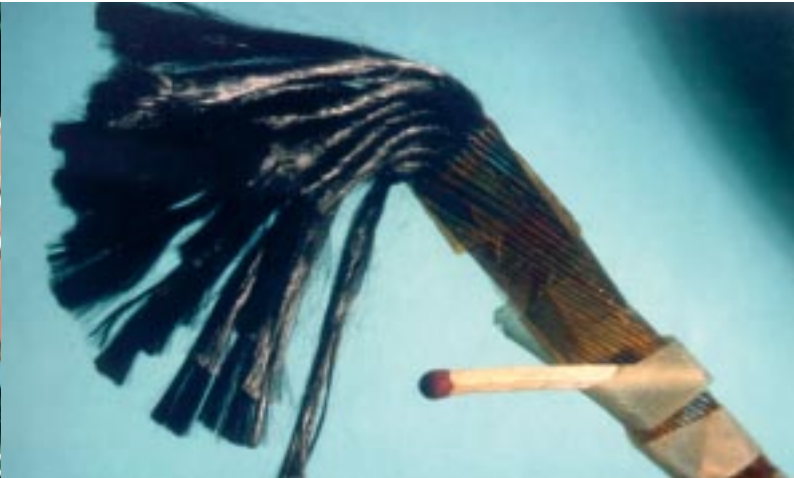
The superconducting cables from which the coils of the proton magnets are wound contain 28 000 filaments.
