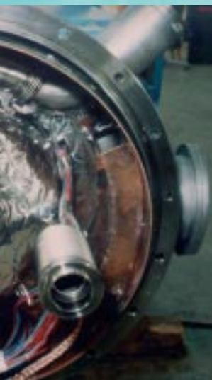
A view into the “head” of a superconducting magnet and the technically complex connections within.
