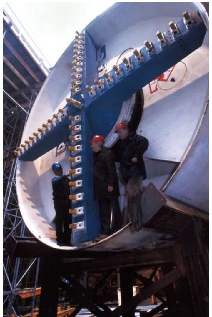
A huge pinion-type cutter: The HERAKLES tunnel boring machine cleared the way for HERA.
