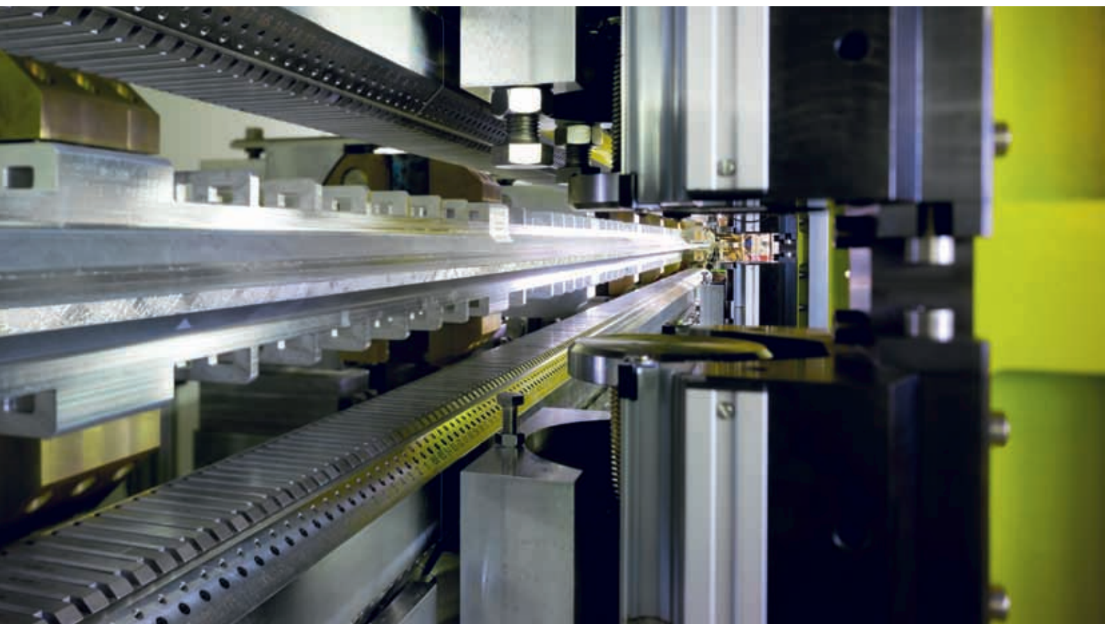
The beam pipe between the magnets of a PETRA III undulator
