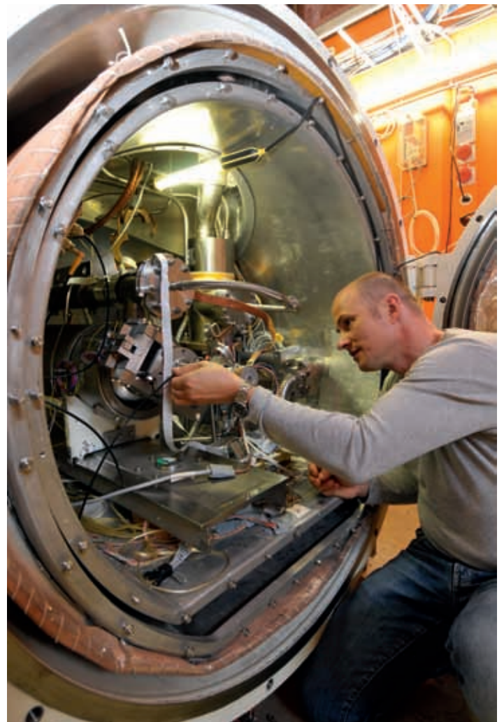
● Preparing for final tests of the superconducting resonators
