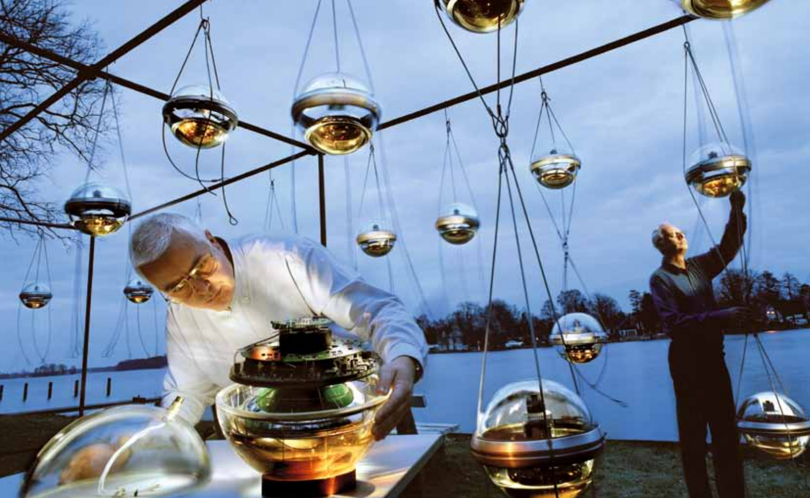
● One quarter of the light sensors for the neutrino telescope IceCube were made at DESY in Zeuthen. The installation in the photograph suggests the geometrical arrangement in which the sensors are frozen, deep in the Antarctic ice.
