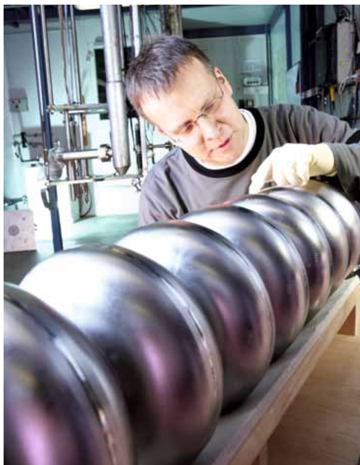
● Inspection of a superconducting niobium cavity at DESY
