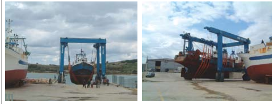
FIGURE 37 Mobile gantry – 250-tonne capacity
