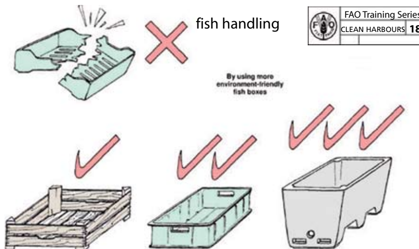
Drawing No.18 suggests more environment-friendly methods of storing fish. Foam and timber boxes accumulate bacteria and are not suitable for continuous use. However, timber boxes are made locally and can be used as fuel when they break.
