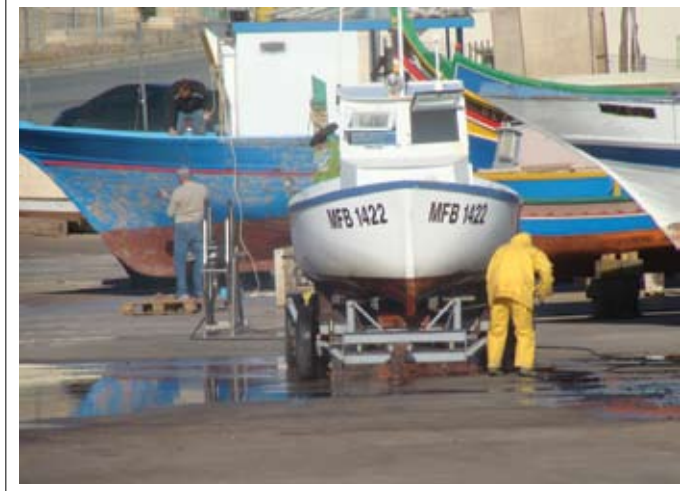
FIGURE 42 Power washing hull
