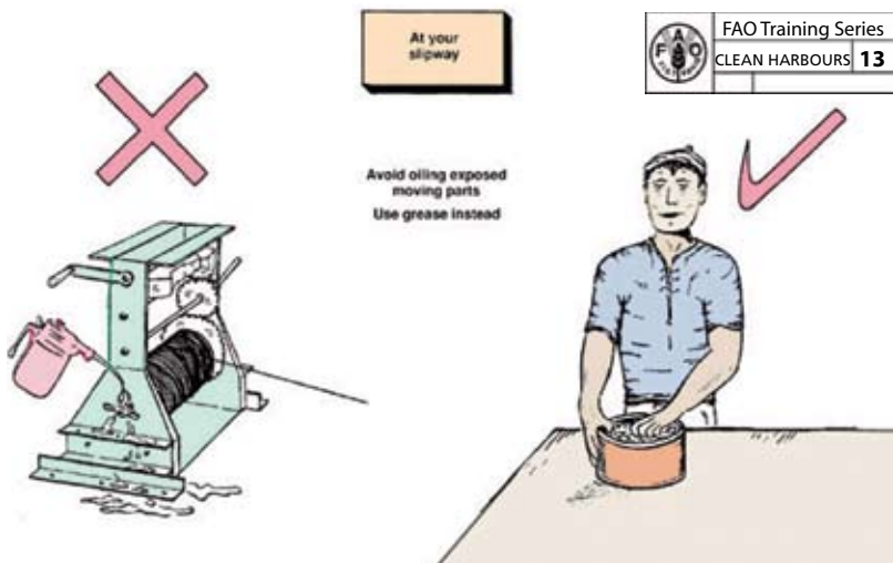
Drawing No.13 explains the importance of greasing moving parts rather than oiling them.
