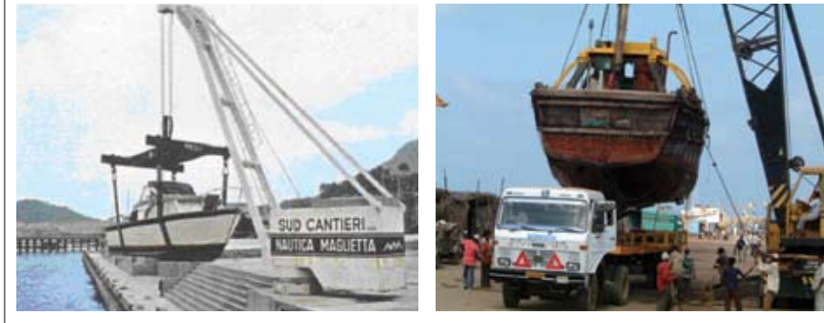
FIGURE 41 Mobile or fixed cranes used to launch or recover vessels
