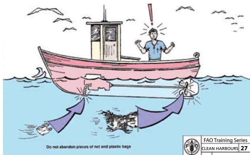
Drawing No. 27 illustrates two cases where such items cause inconvenience to other vessels.
