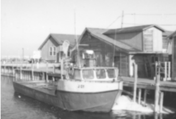
Figure 4—The Joy , which works out of Leland, Michigan, is typical of the trap net boats that are used on Lake Michigan today. Its long, open stern area allows for the safe and manageable retrieval of the trap net's pot section—the end of the net and the main entrapment device on this type of harvesting technology. The trap net is essentially a submerged version of a pound net. (Photograph by Chiarappa)
