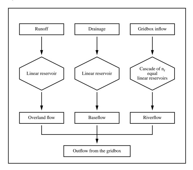
Fig. 1: Structure of the HD model
