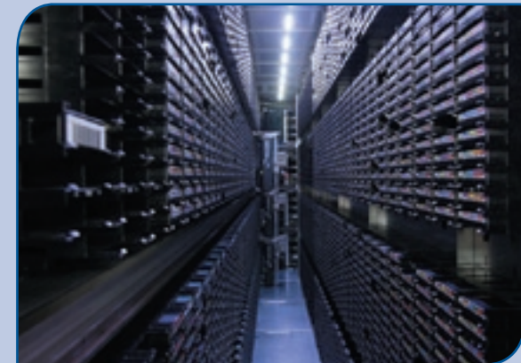
View into the interior of one of the DKRZ's tape libraries showing hundreds of data cartridges
