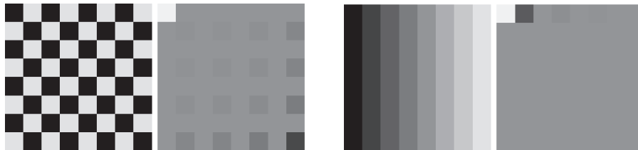
Figure 3: Checker and gradient pattern and their DCTed equivalents
